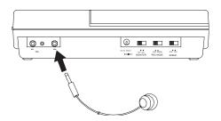
**Note:** The speaker automatically disconnects when you plug in an earphone.
